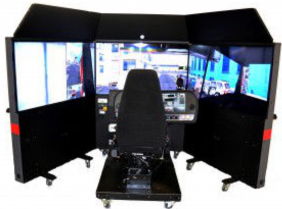
The DriveWise VS6 Driving Simulator used by Uxbridge Firefighters to train on defensive and emergency driving
