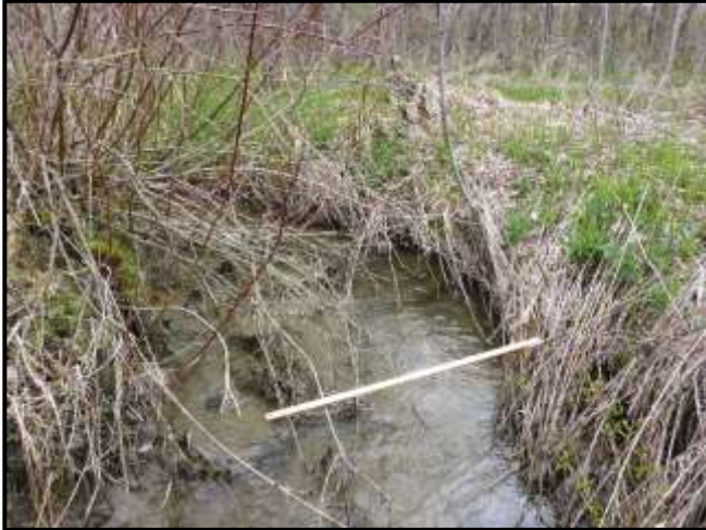
Photograph 9. Reach UBT-1 Upstream view of basal scour along both inner and outer banks at meander bend.
