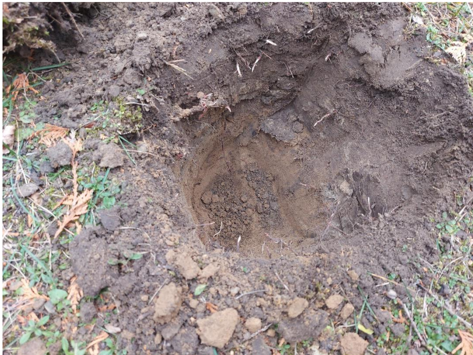
Image 20: Open Test Pit showing Subsurface Stratigraphy
